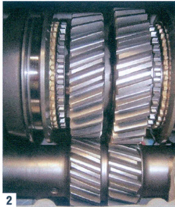
2 The M-22 gearset with its distinctive 20-degree helix angle on the teeth.
