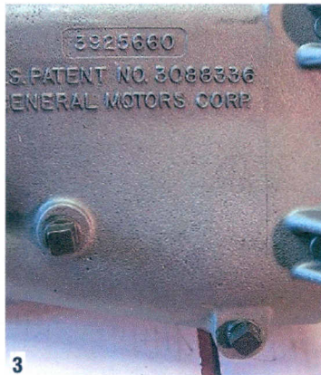
3 An M-22 case with the drain plug in the boss at the bottom; many M-20/21 cases have had this feature added during rebuilds.
