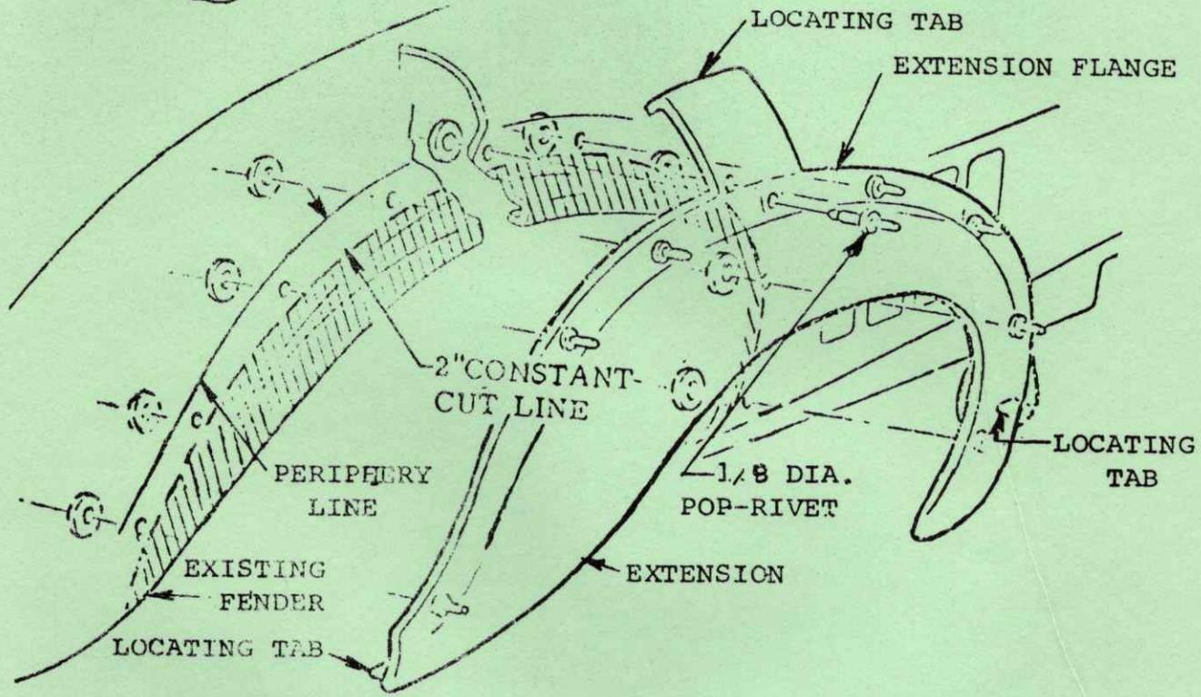
Locate Fender Extension Tabs on body, use extension as template to mark periphery.
