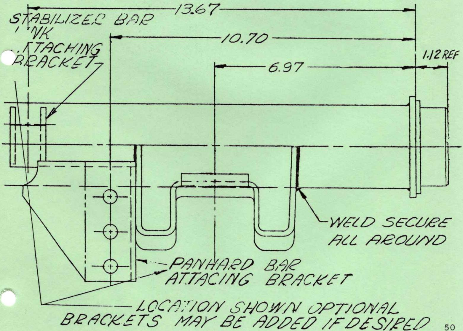
**NOTE** Bend sheet metal flange for this distance to provide clearance for stabilizer in full jounce.
