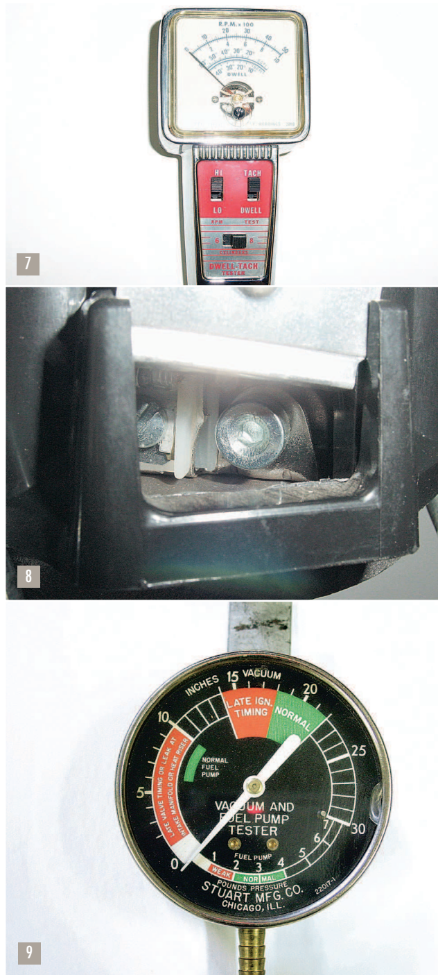
7 I’ve had this dwell/tach meter for 30 years. Actron, Sears, and others have similar meters today for $25-$50.
