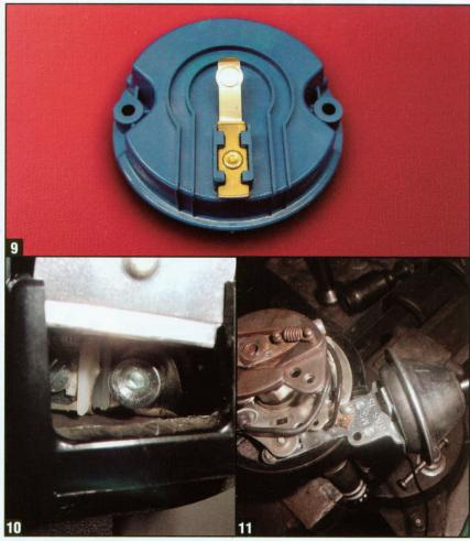
**9** The rotor attaches to the centrifugal advance mechanism, and transfers high-voltage current from the center of the cap to the plug wire terminals.
