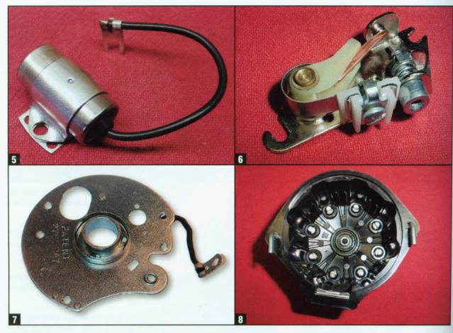
5 The condenser, which assists in the rapid collapse of the coil's magnetic field and minimizes arcing and pitting of the points.
