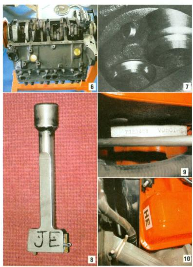
6 The timing cover, harmonic damper, and oil pump were added just prior to oil pan installation. Photo Dave McDufford
