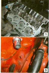
1 The bare block looked like this when it came off the machining line and emerged from the high-pressure washer, ready for assembly.
