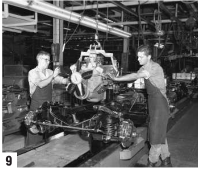
9 A 1966 L-79 engine positioned for drop on the chassis line. Note shim count markings at the front of the frame horn. (GM Photo)
