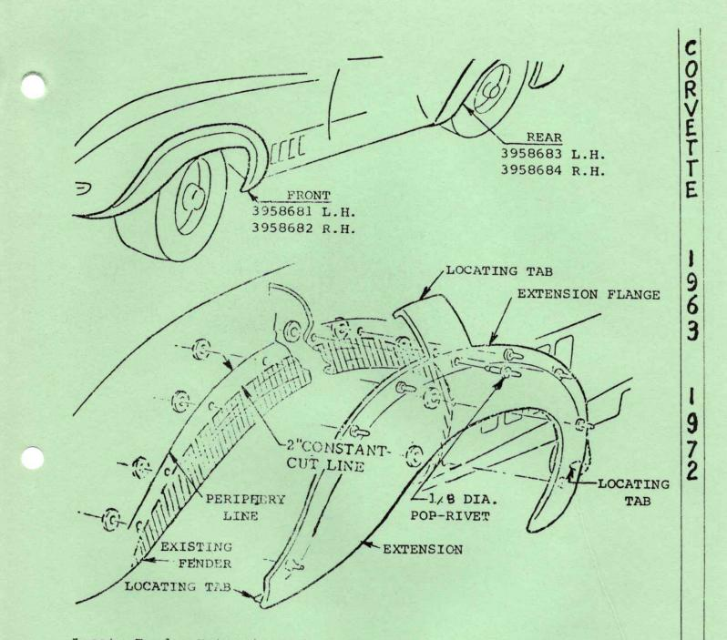
Locate Fender Extension Tabs on body, use extension as template to mark periphery.
